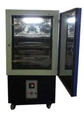
The BOD incubator is most versatile and highly reliable low temperature incubator to make Biochemical Oxygen Demand determinations and for preservation of vaccines, insulin, level extracts, chemicals etc.
